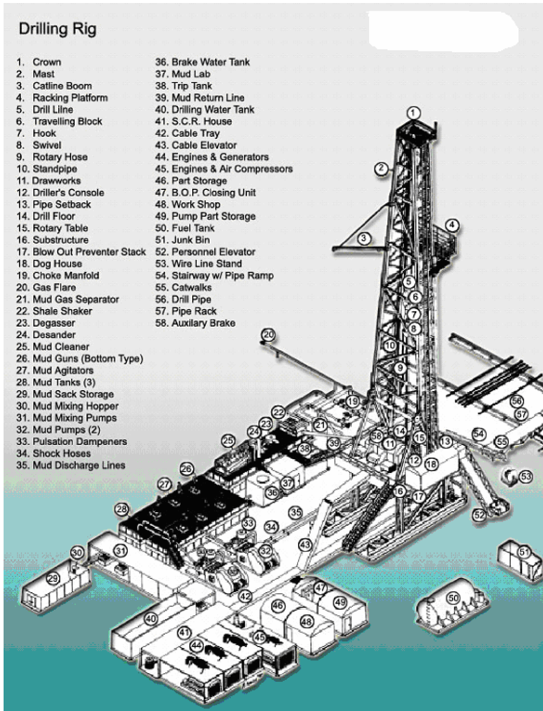
Figure 2.1. Typical Land Drilling Rig
