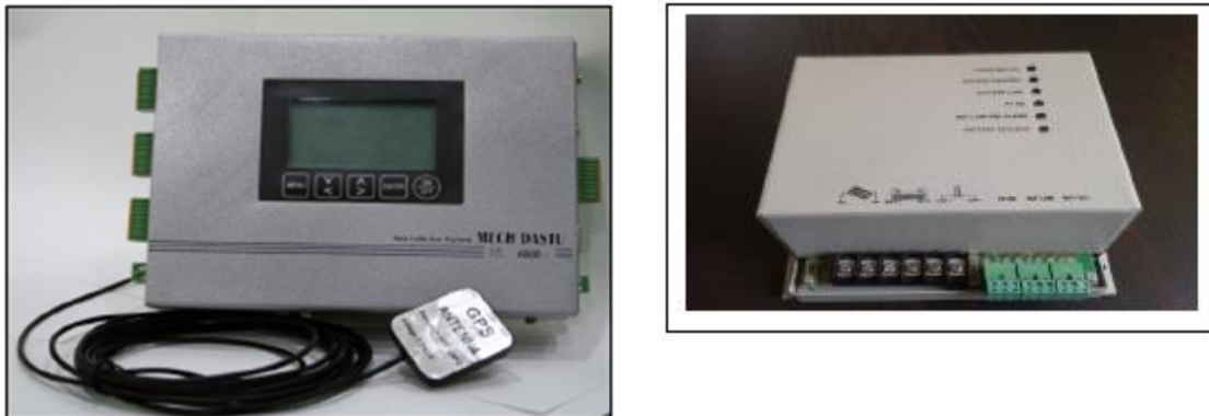
Figure 9-6: Typical data collection platform and online battery charger
